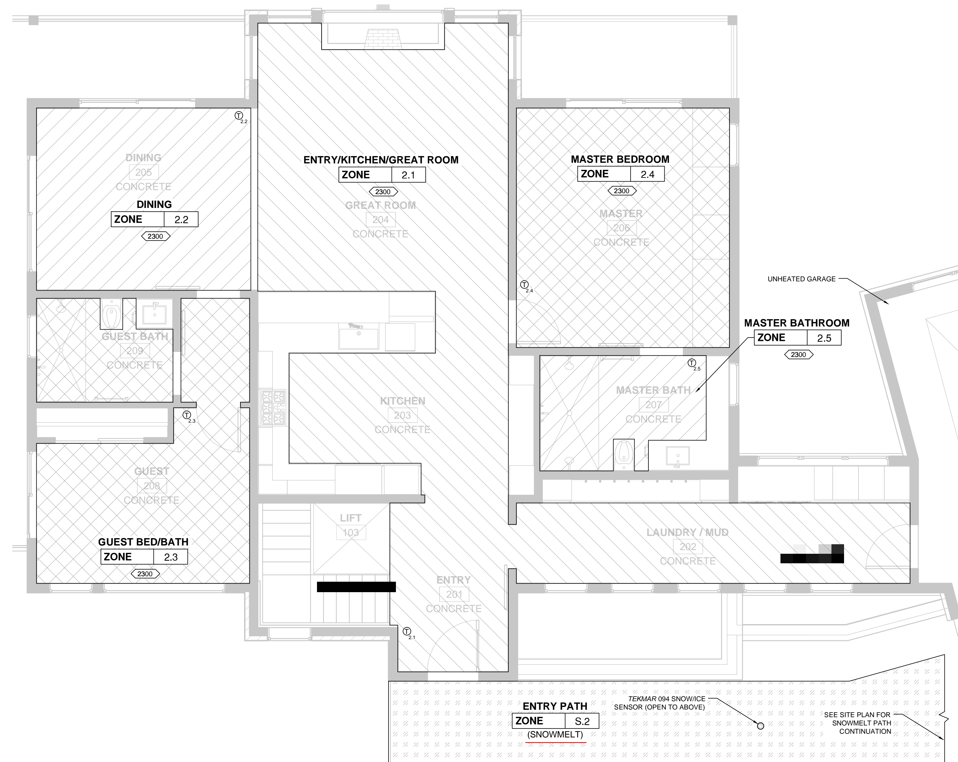
3 GROUND LEVEL HYDRONIC HEATING SCALE: 1/4" = 1'-0"
