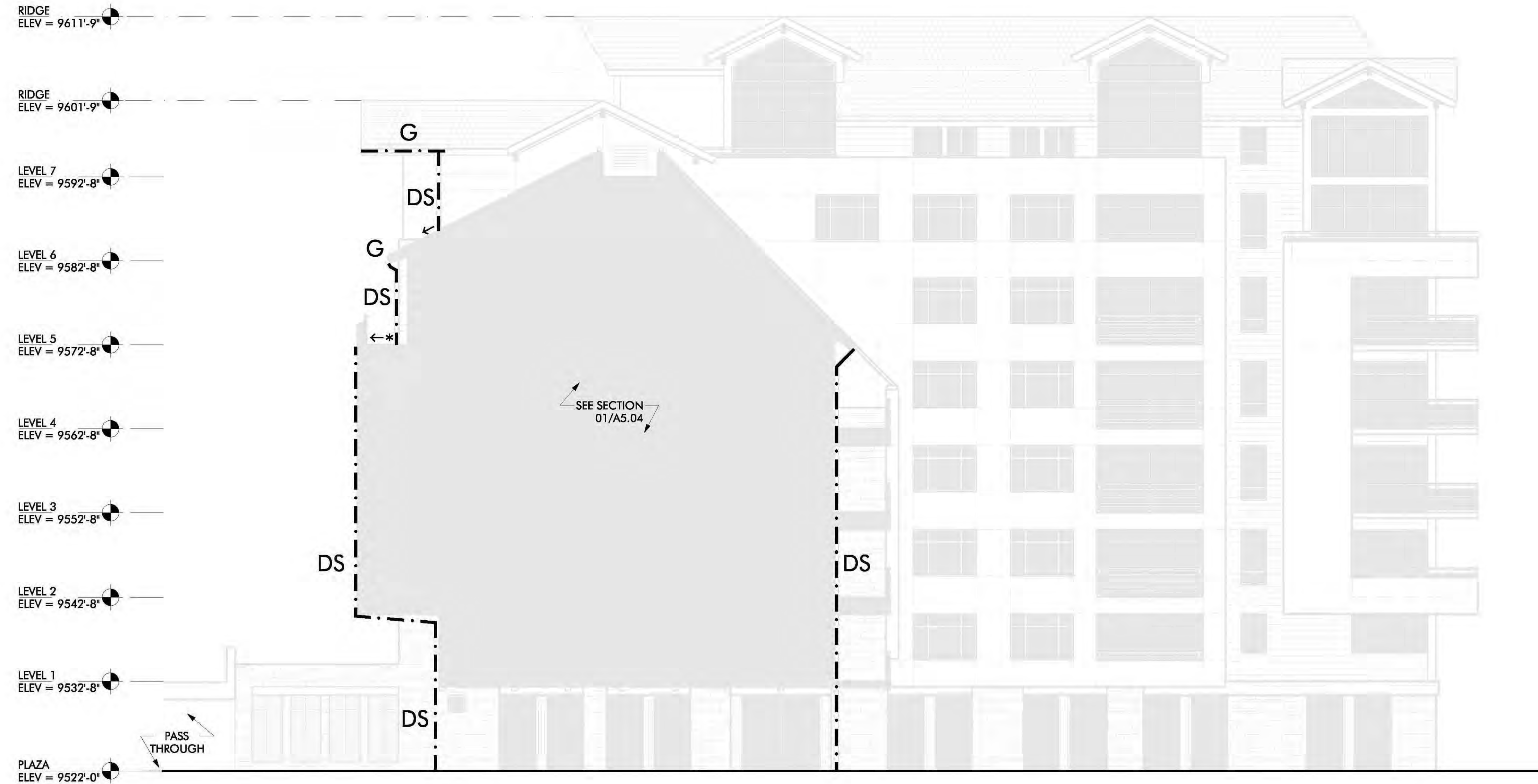
01 NORTH BREEZEWAY ELEVATION LOOKING WEST SCALE: 1/8" = 1'-0"
