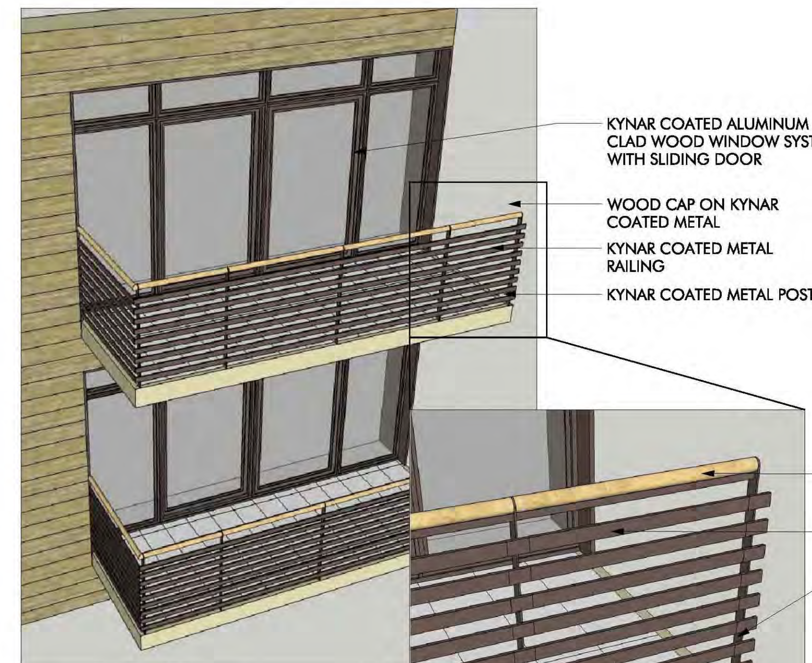
06 TYPICAL WINDOW IN WOOD SIDING SCALE: NO SCALE
