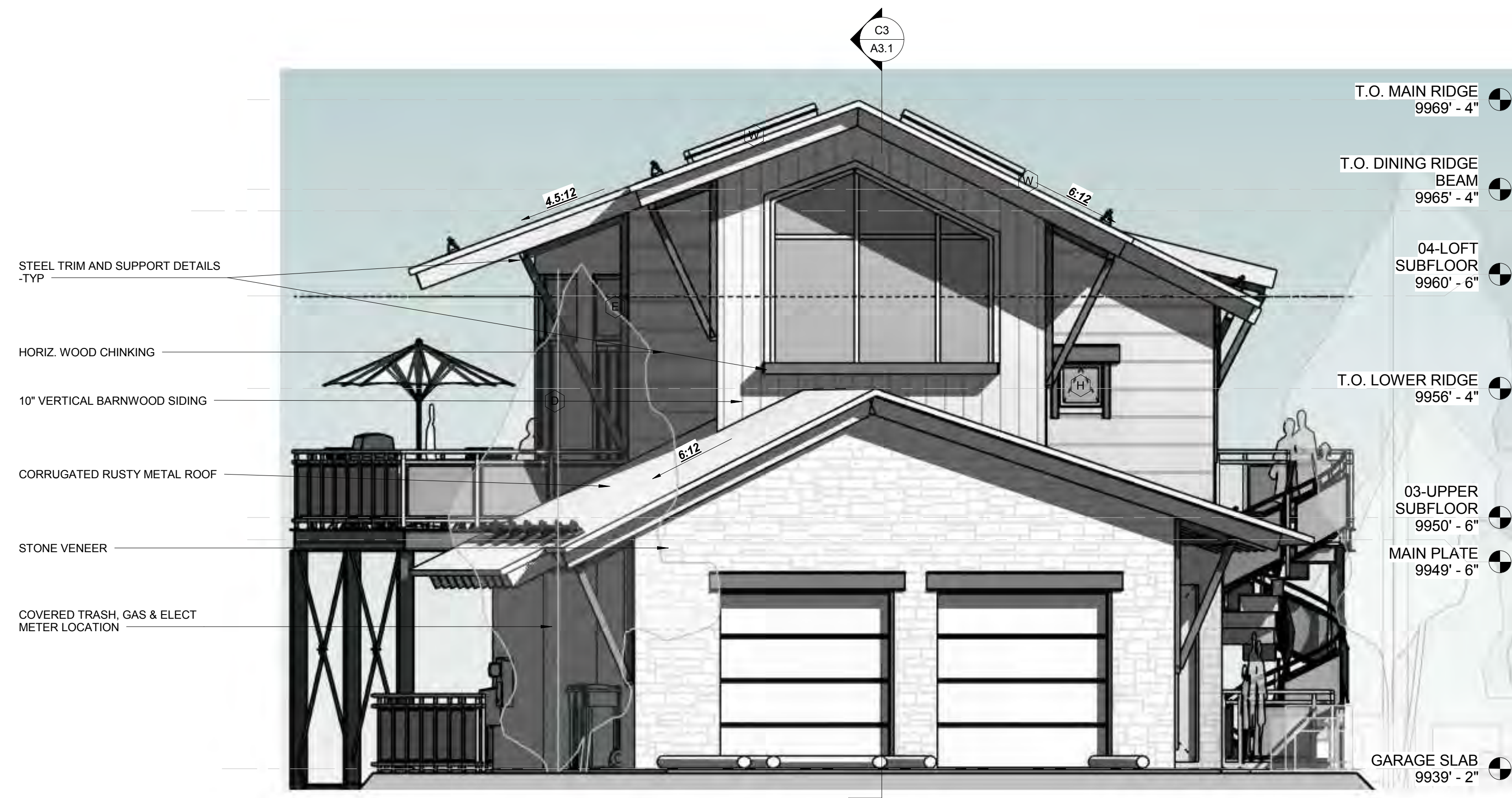
A1 WEST (CABINS LANE) ELEVATION 1/4" = 1'-0"
