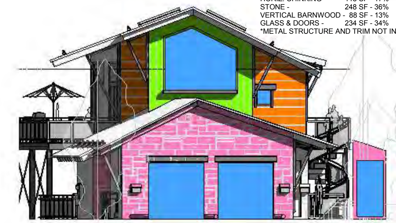
A3 WEST ELEVATION MATERIALS 1/8" = 1'-0"
