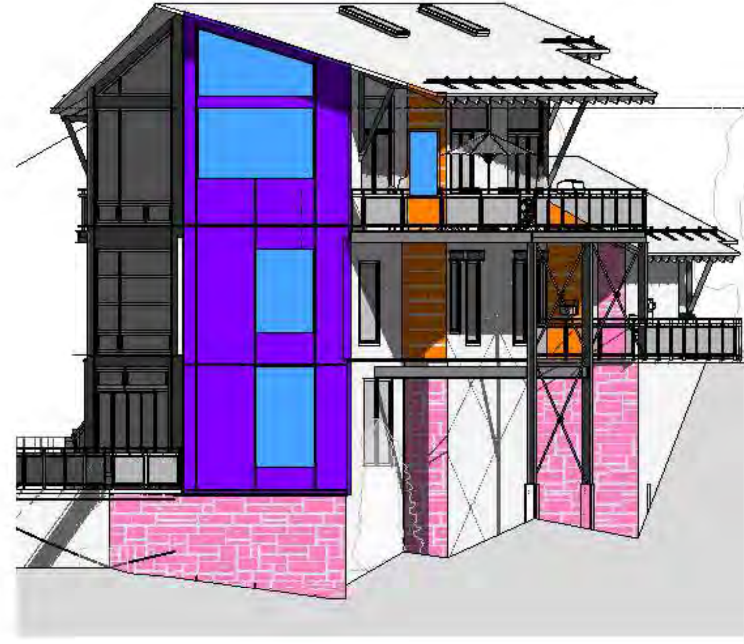
C2 NORTHEAST ELEVATION MATERIALS 1/8" = 1'-0"
