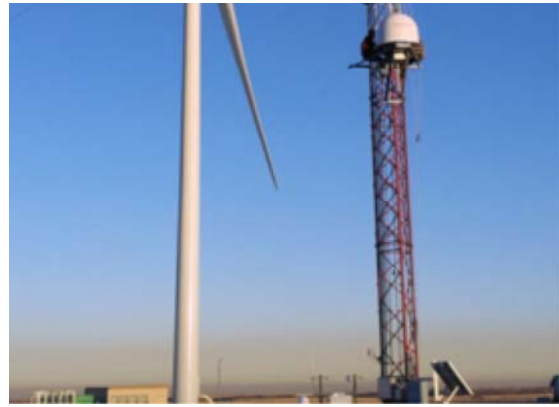
MD-12 radar system installed at NREL
