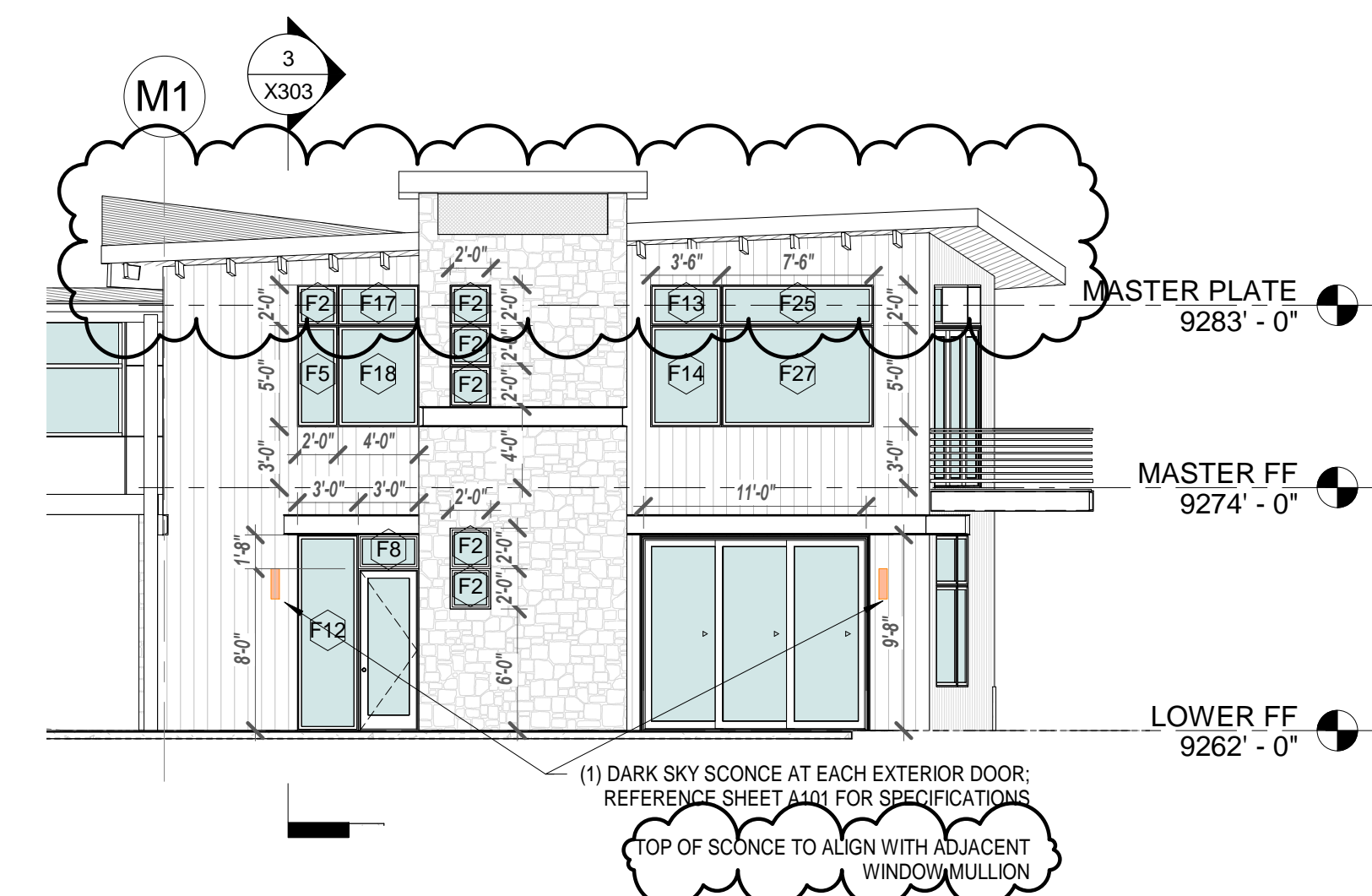
5 ELEVATION - MASTER EAST 1/8" = 1'-0"
