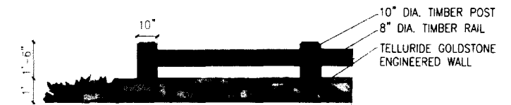
ELEVATION C - 30" GUARD RAIL (5' MIN. DISTANCE FROM TRAIL)
