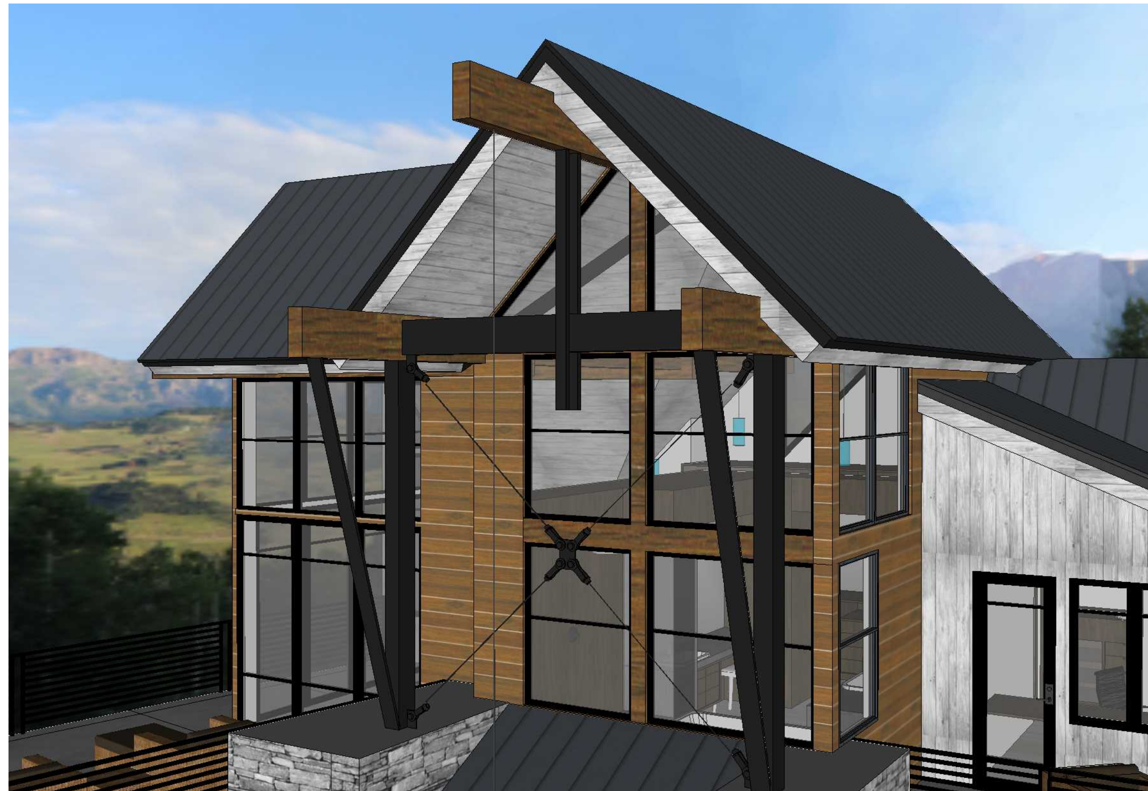
GABLE CROSS-BRACKET DETAIL
