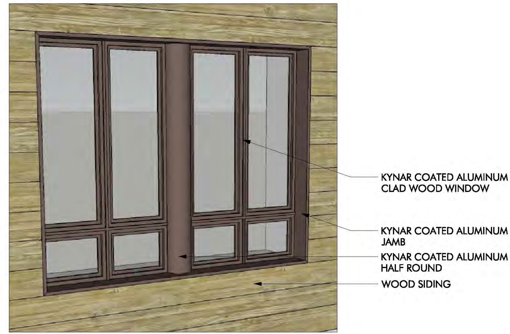
06 TYPICAL WINDOW IN WOOD SIDING SCALE: NO SCALE
