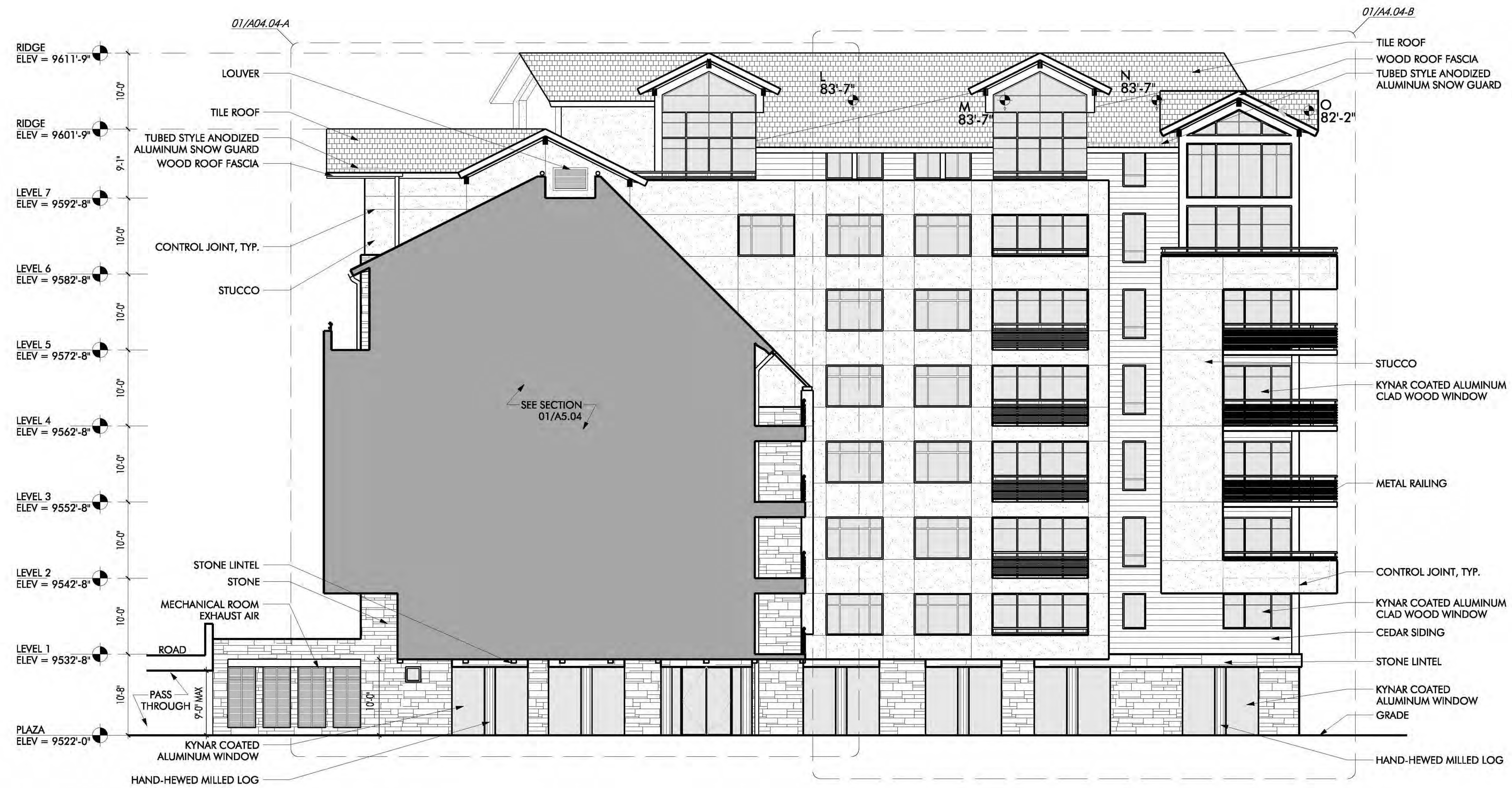
01 NORTH BREEZEWAY ELEVATION LOOKING WEST SCALE: 1/8" = 1'-0"
