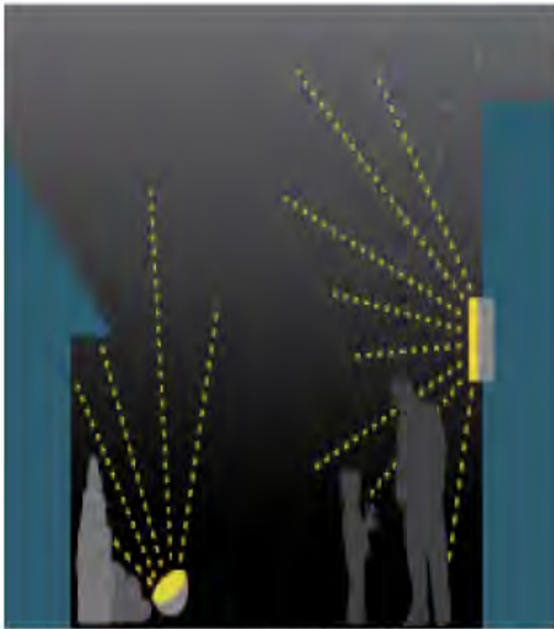
Unshielded fixtures create glare and waste light.
