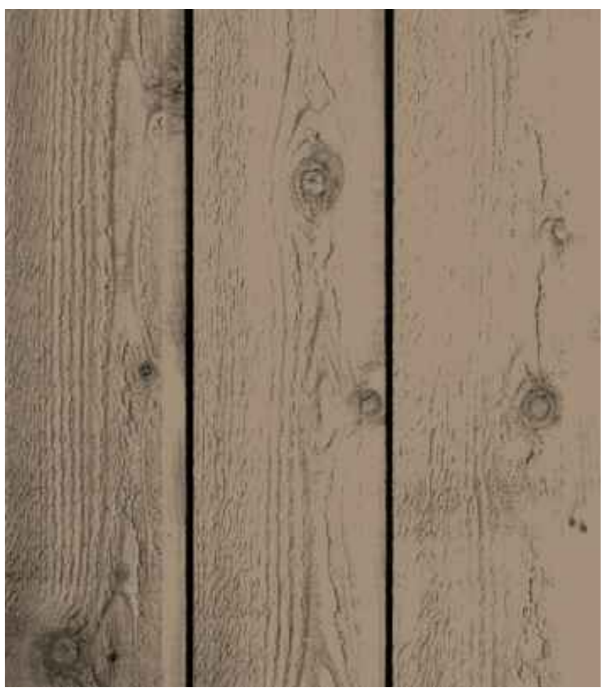
8" FIRE TREATED, STAINED, CHANNEL RUSTIC CEDAR SIDING COLOR: BEECHWOOD GRAY, SEMI TRANSPARENT MANUFACTURER: CABOT
