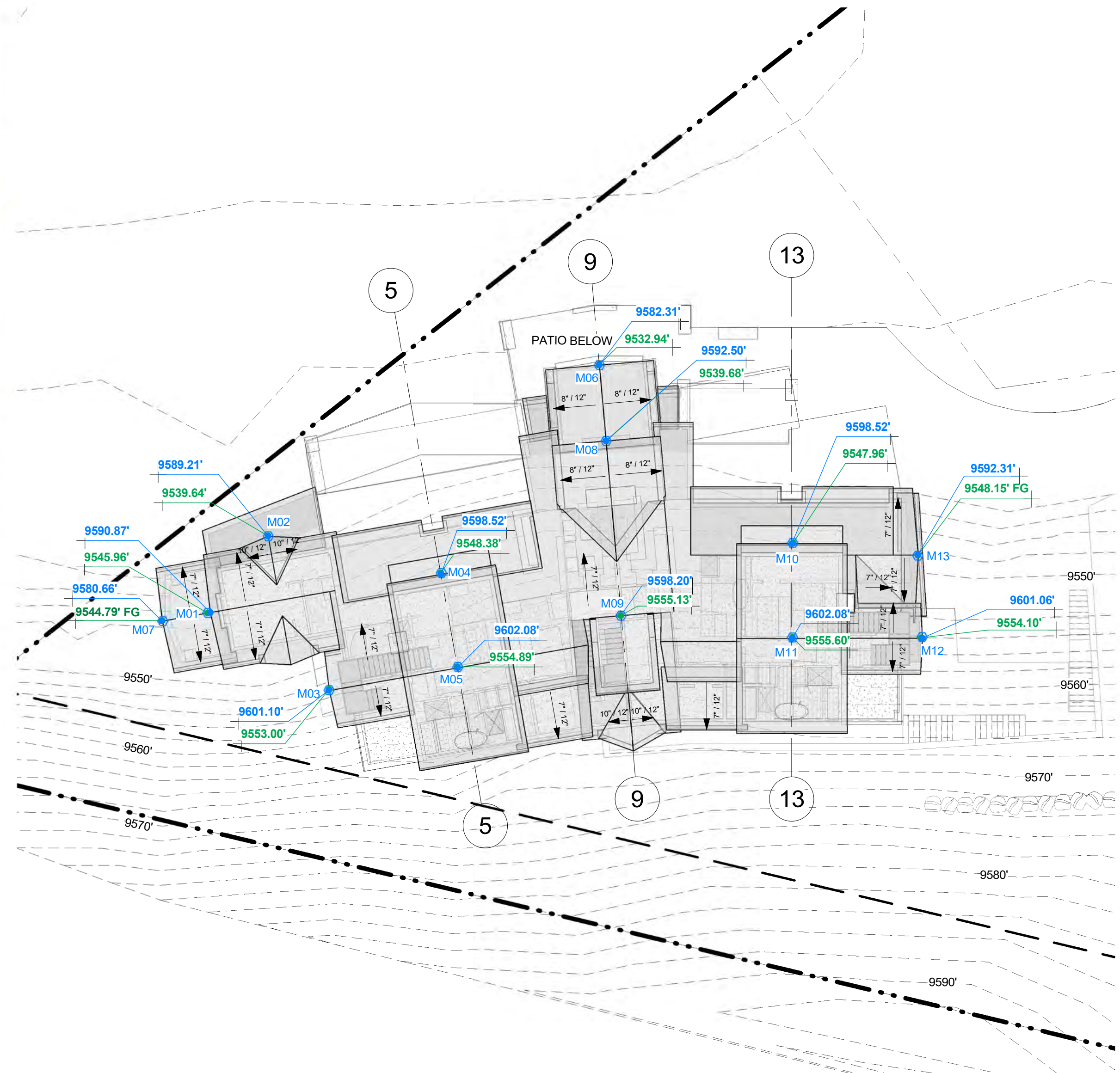
2 ROOF HEIGHT POINTS PLAN - MAXIMUM HEIGHTS H1.00 1/16" = 1'-0"
