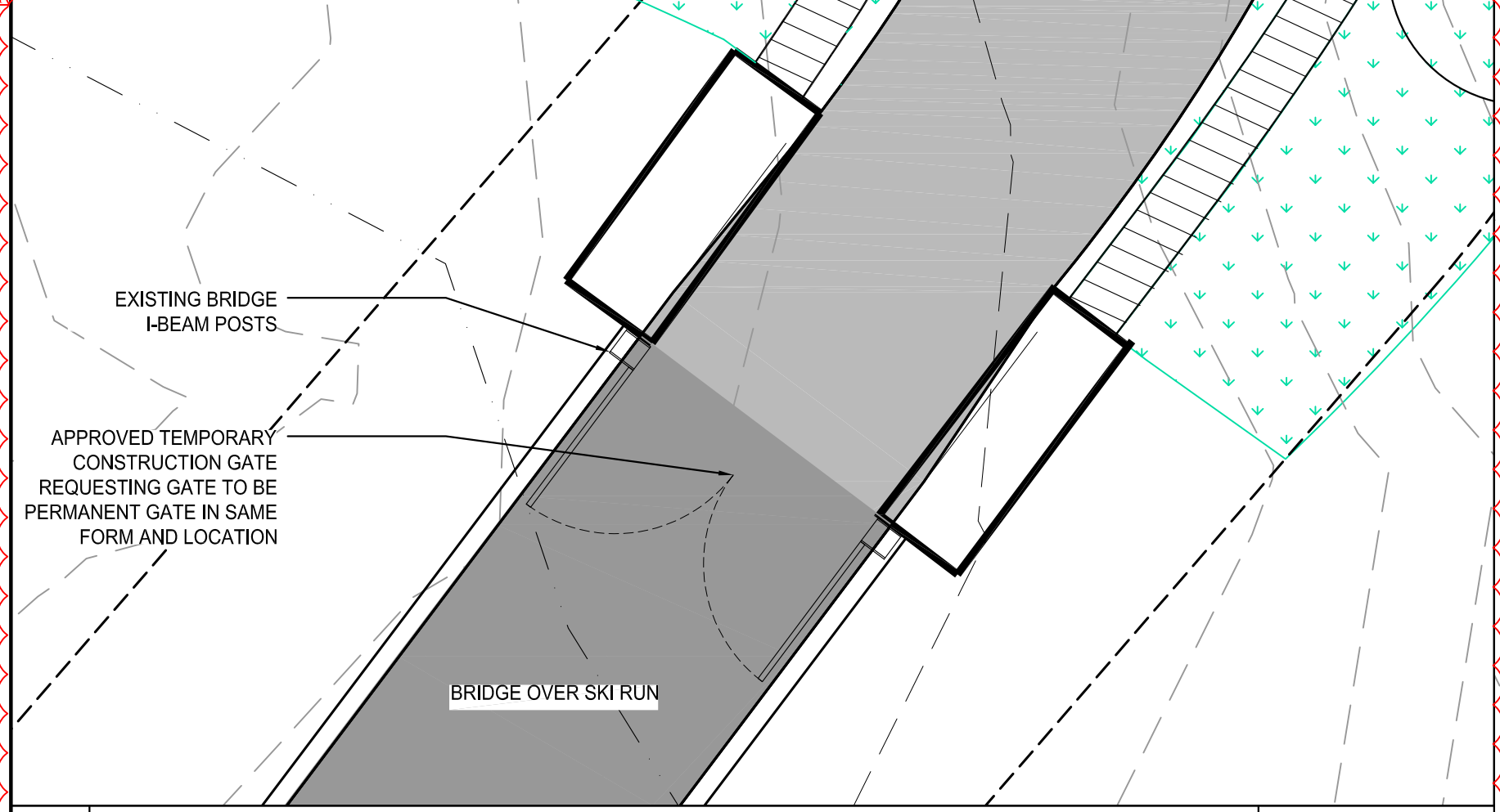
3 ENLARGED PLAN @ GATE SCALE 1/8"=1'-0"
