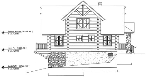
CABIN TWO LEFT SIDE ELEVATION Scale: 1"=8'
