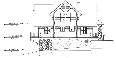
CABIN SEVEN LEFT SIDE ELEVATION Scale: 1"=8'
