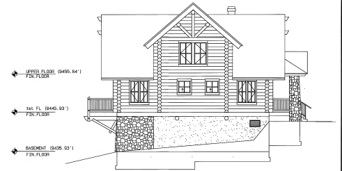
CABIN EIGHT LEFT SIDE ELEVATION Scale: 1"=8'
