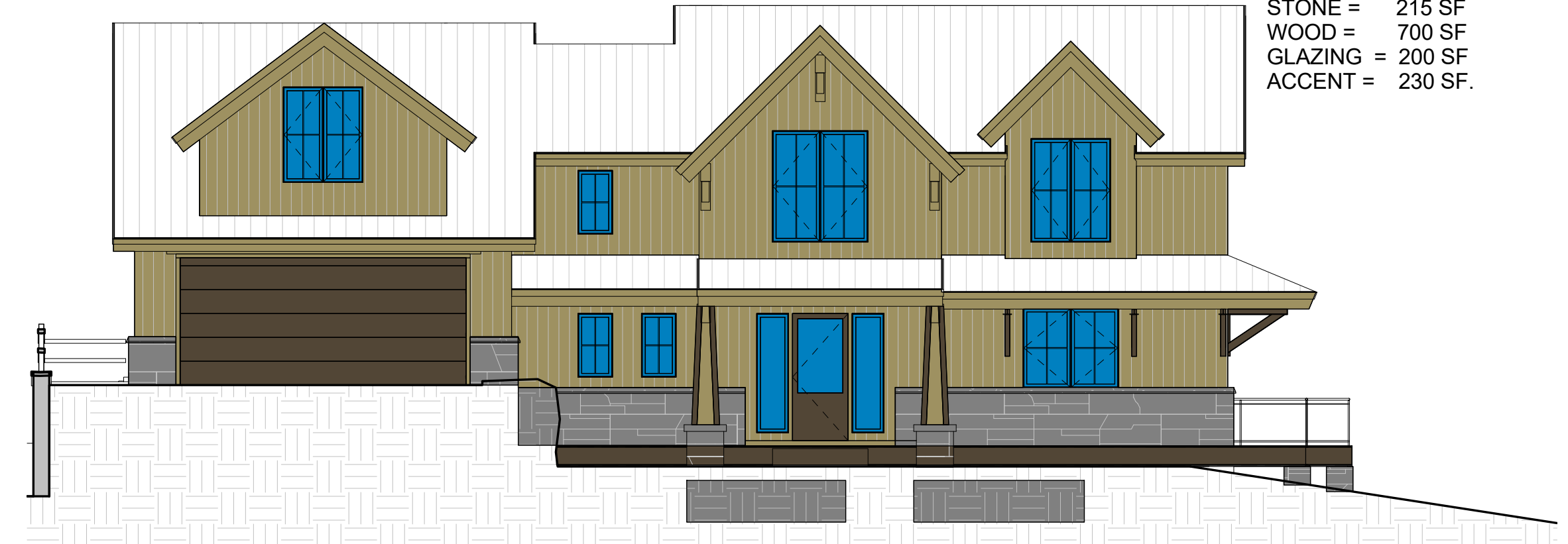
1 MATERIAL CALC 1 SOUTH ELEVATION 1/8" = 1'-0"
