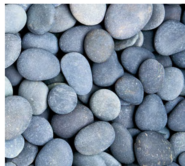
Ballast Roof - Mexican Beach Pebbles
