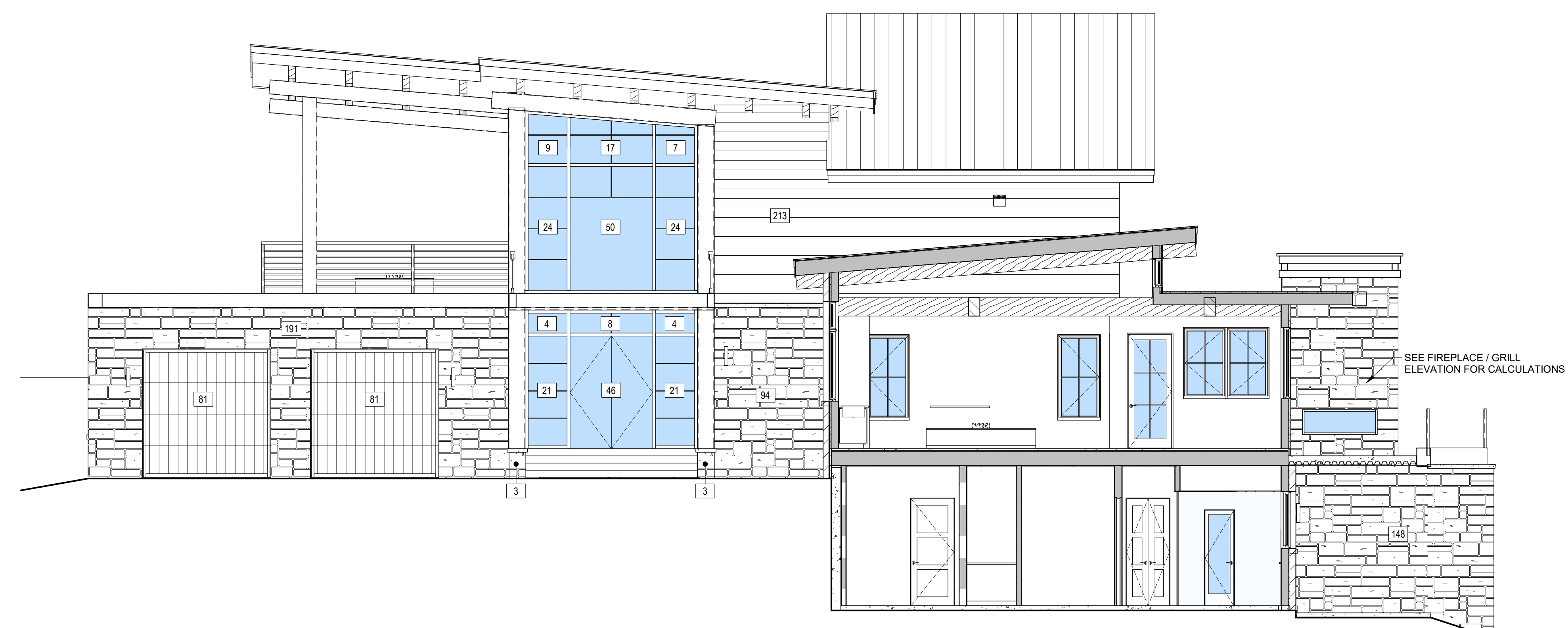
3 WEST ELEVATION AT MASTER 3/16" = 1'-0"
