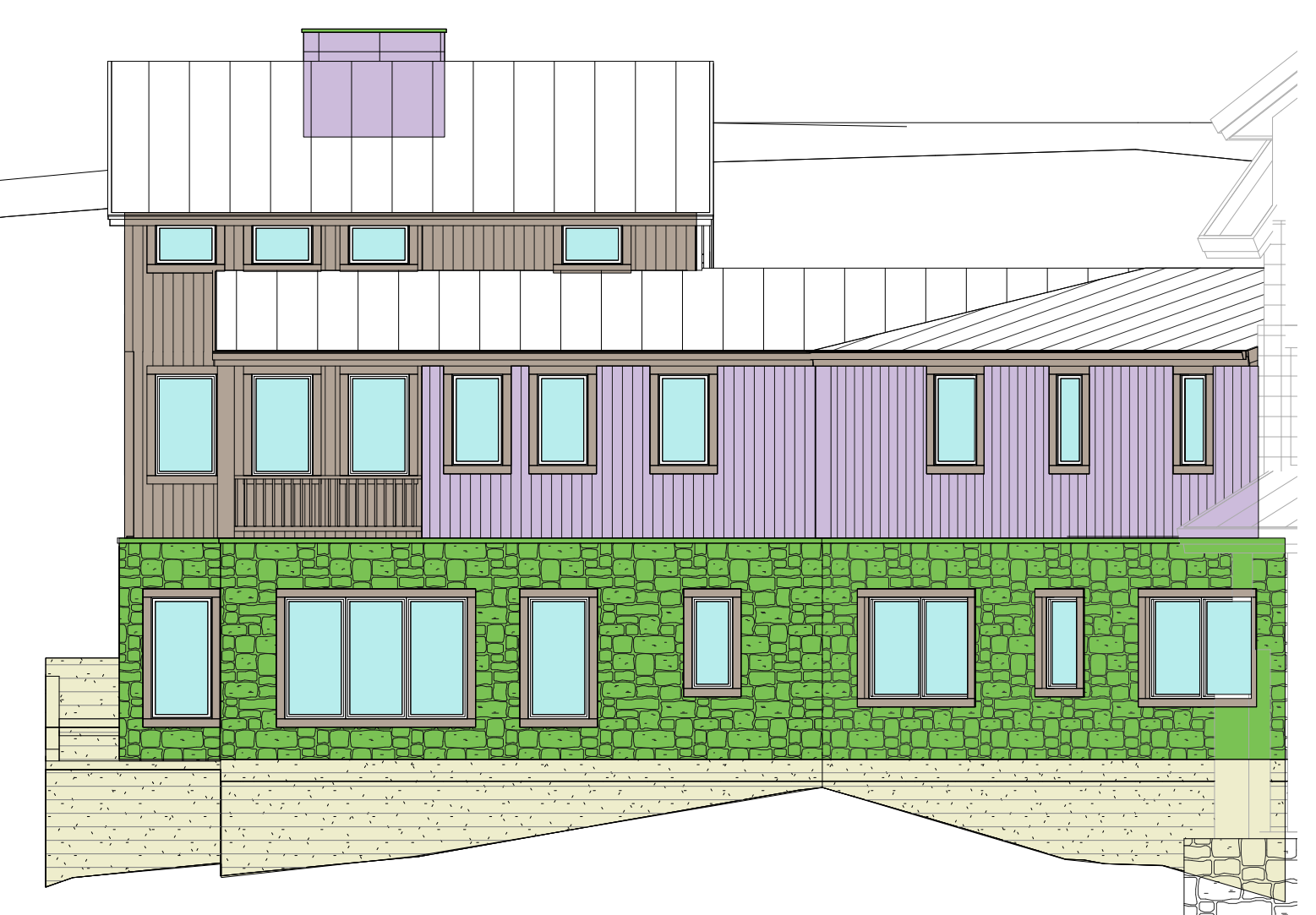
5 Materials - West Elevation
