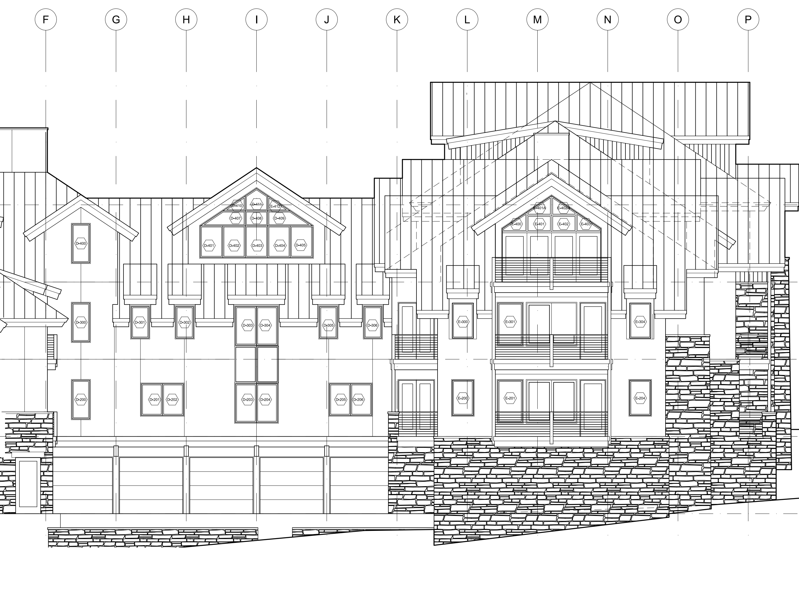
2 ELEVATION - D (WEST) A2.2 1/8"=1'-0"
