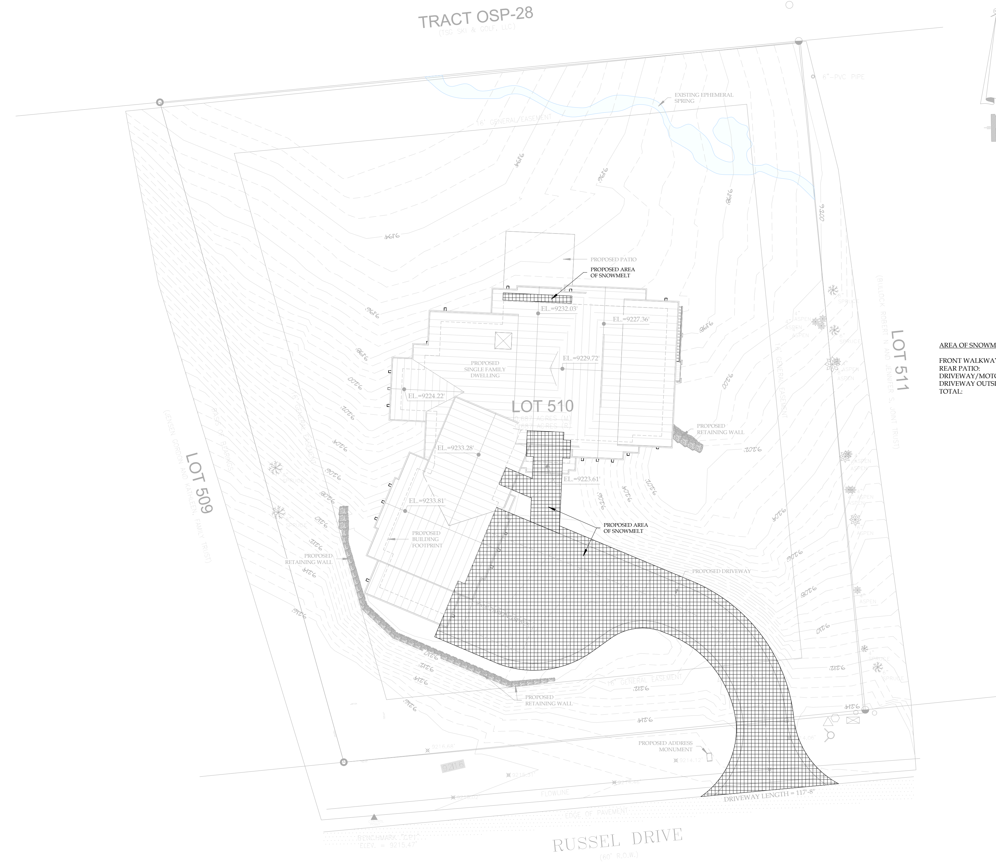
1 SITE PLAN-PROPOSED SNOWMELT AREA 1" = 16'-0"
