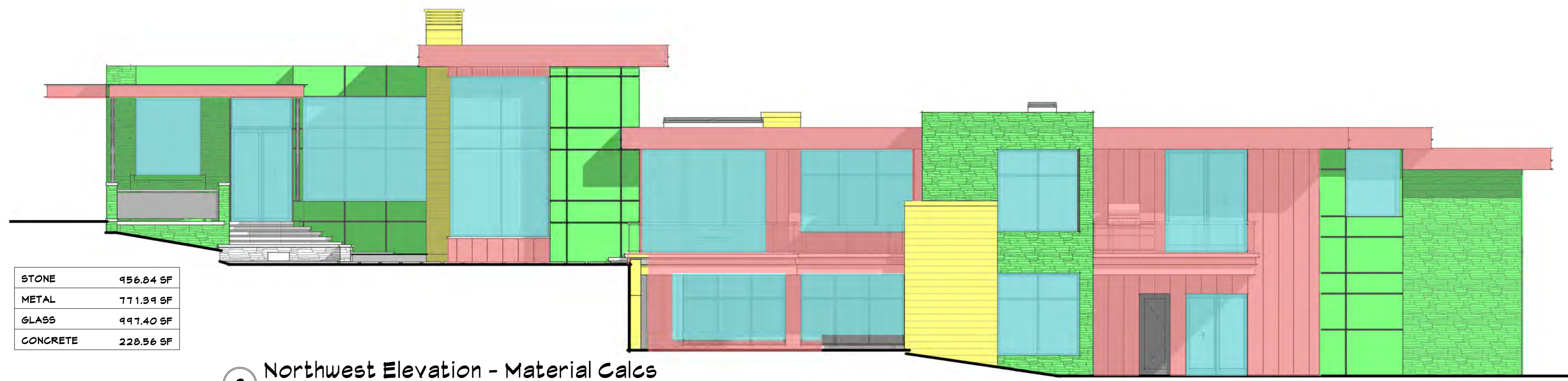
2 Northwest Elevation - Material Calcs
