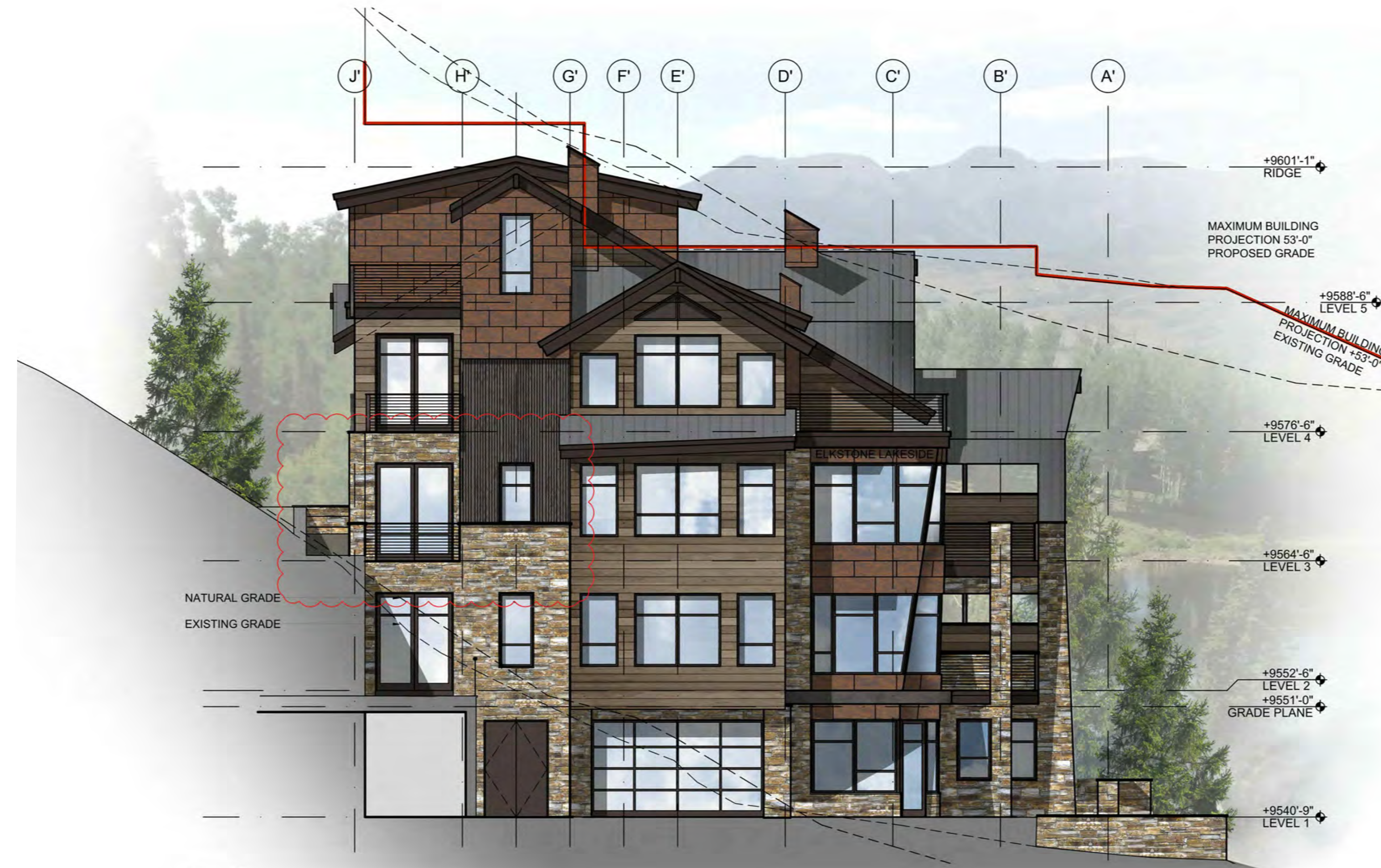
2 EAST ELEVATION (ENTRY) A2.01 1/8" = 1'-0"
