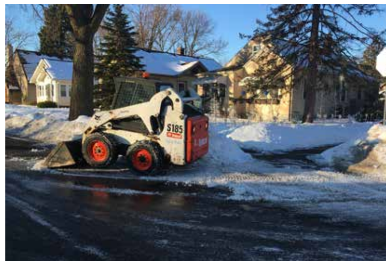
A bobcat with a plow can be used to plow shared use paths and sidepaths.
