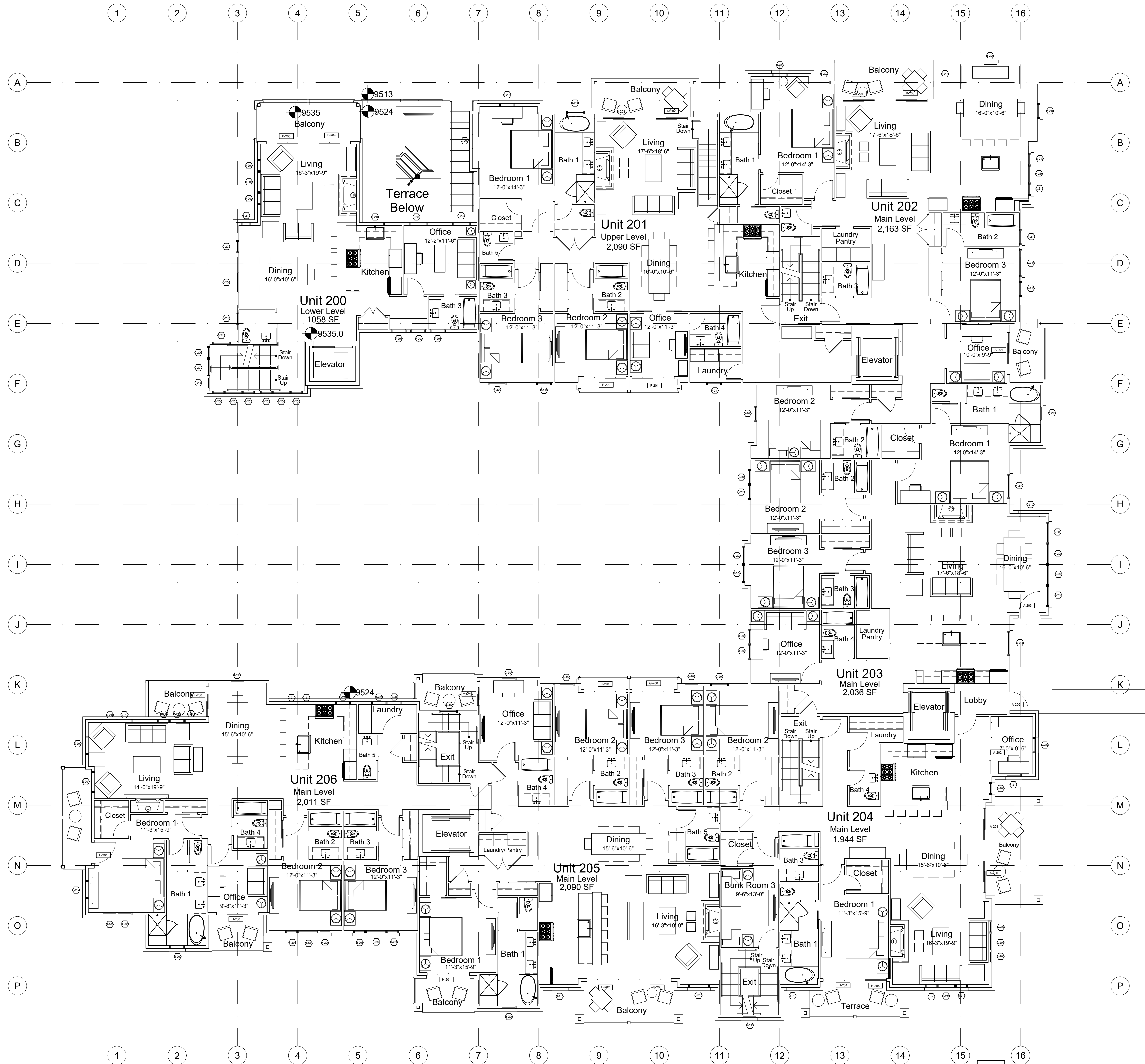
1 LEVEL 02 FLOOR PLAN (+935.0) A1.3 1/8"=1'-0"
