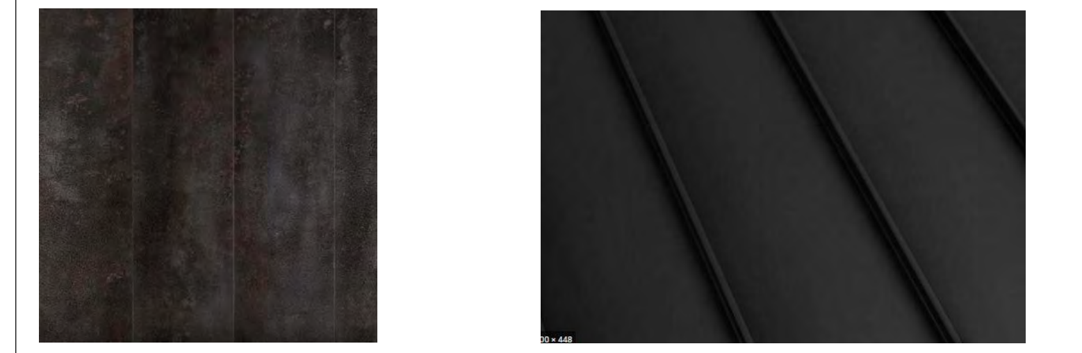
BLACKENED STEEL METAL PANEL SYSTEM DARK PREFINISHED METAL ROOF WILL BE EITHER A DARK STEEL OR ZINC PER 17.5.6.C.3.C.iv DARK PREFINISHED ALUMINUM SHEET METAL AT WINDOWS (NON REFLECTIVE) TO MATCH THE ROOF
