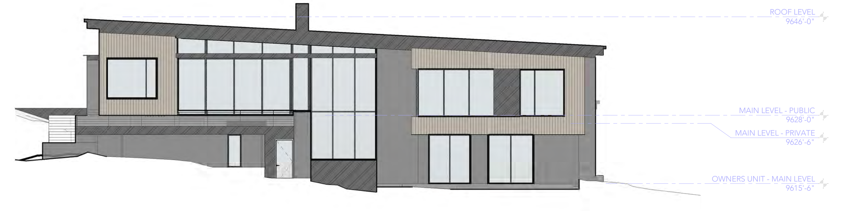
NORTH ELEVATION | 2 3/32" = 1'-0" NORTH ELEVATION MATERIAL AREAS: STONE: 691 SF WOOD: 367 SF METAL: 446 SF GLAZING: 922 SF - 38% TOTAL: 2,426 SF
