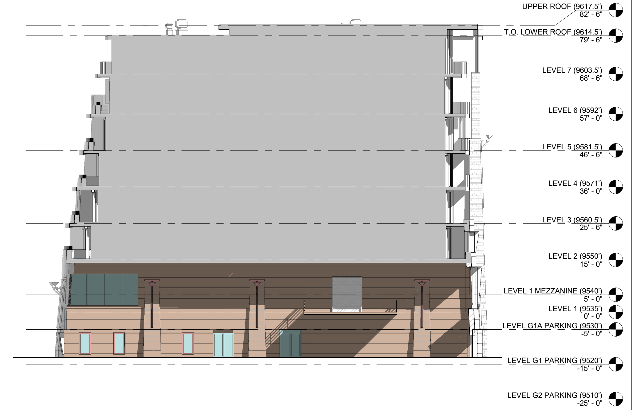
EXTERIOR ELEVATION - MATERIAL - PEDESTRIAN WEST 1/16" = 1'-0"
