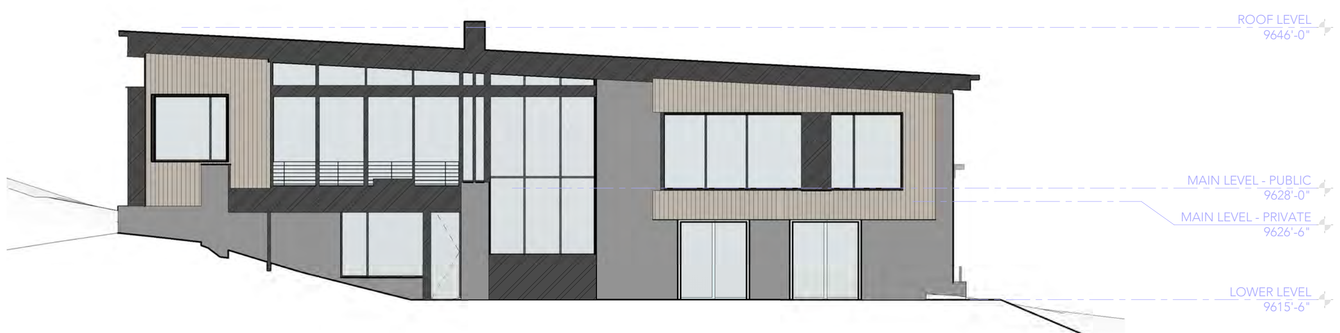
NORTH ELEVATION | 2 3/32" = 1'-0" NORTH ELEVATION MATERIAL AREAS: STONE: 551 SF WOOD: 368 SF METAL: 525 SF GLAZING: 947 SF - 39.6% TOTAL: 2,391 SF
