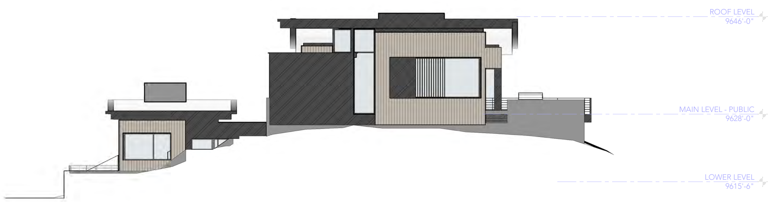
EAST ELEVATION | 1 3/32" = 1'-0" EAST ELEVATION MATERIAL AREAS: STONE: 186 SF WOOD: 305 SF METAL: 450 SF GLAZING: 233 SF - 19.8% TOTAL: 1,174 SF
