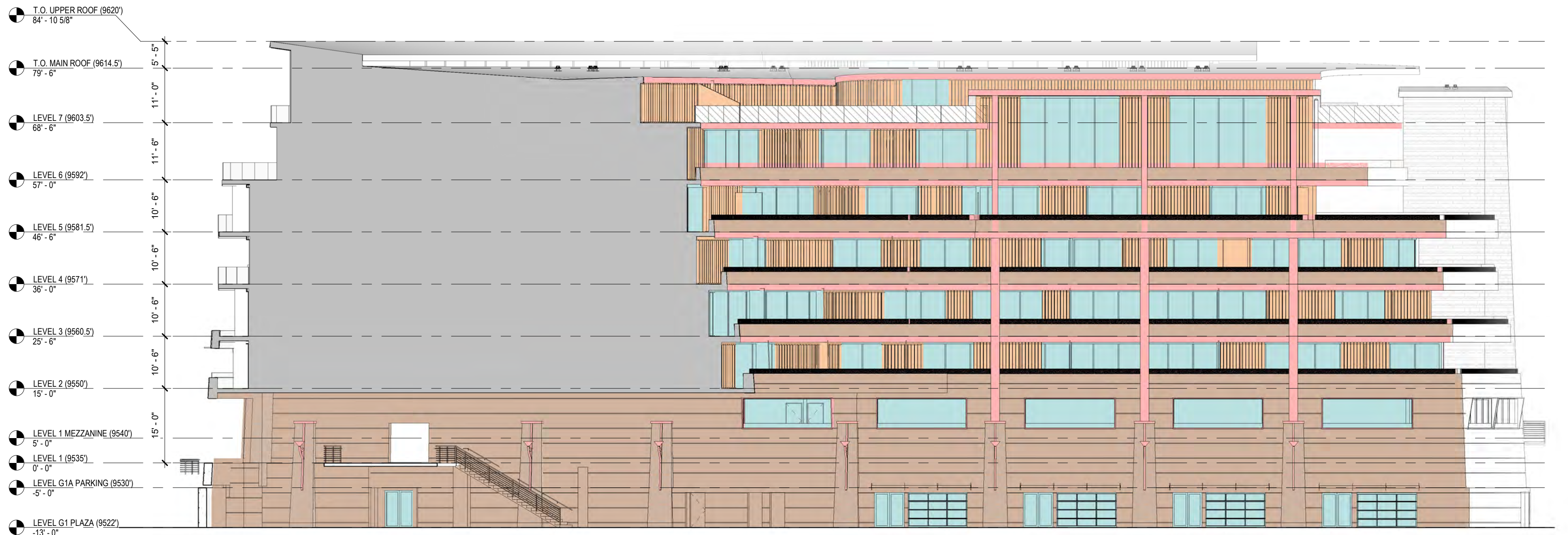
1 MATERIAL ELEVATION - SOUTHEAST 1/16" = 1'-0"
