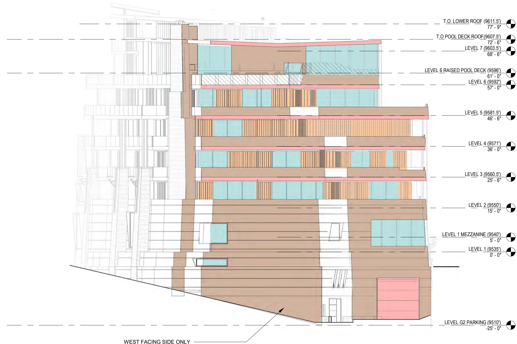
5 WEST MATERIAL ELEVATION 1/16" = 1'-0"
