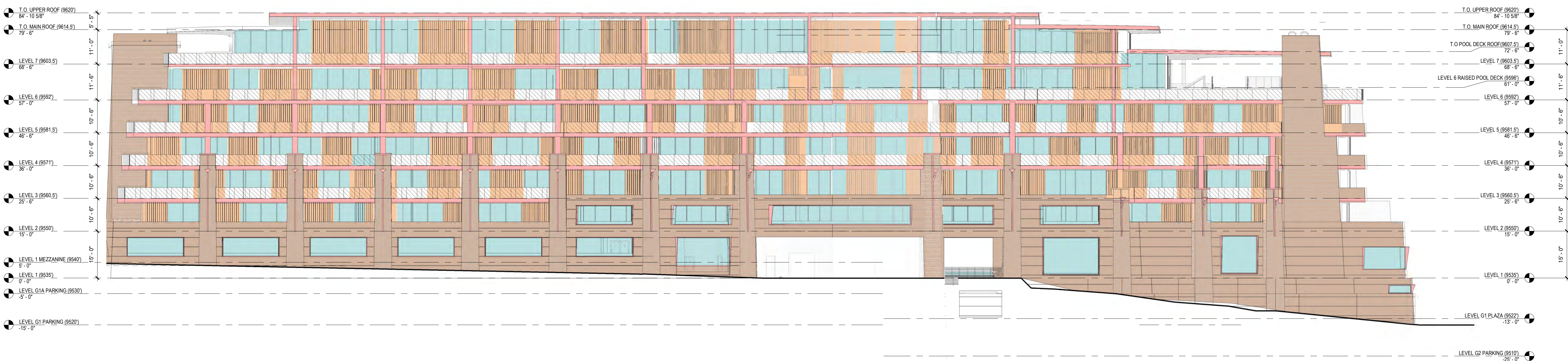
1 NORTHEAST MATERIAL ELEVATION 1/16" = 1'-0"
