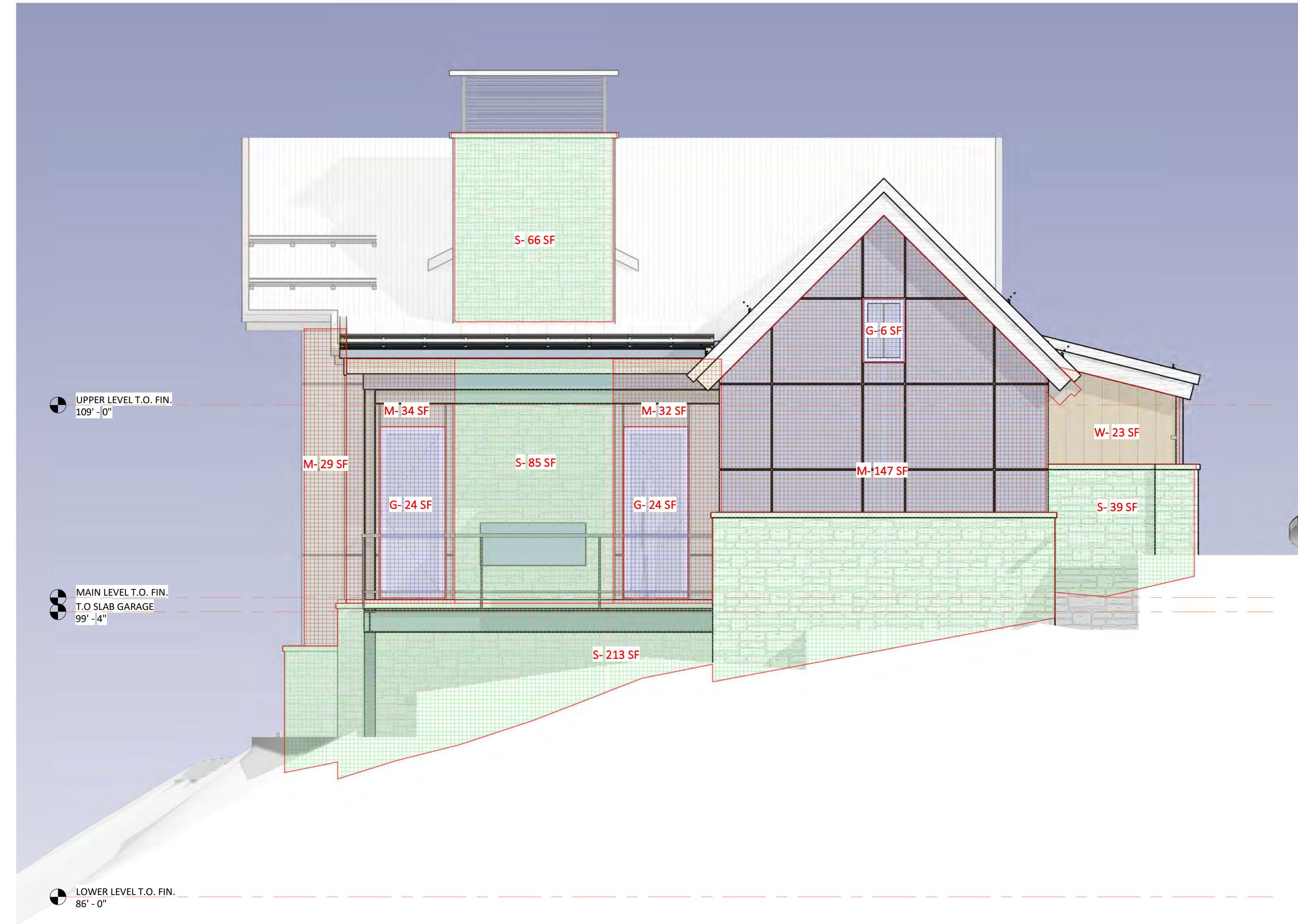
1 MASTER EAST ELEVATION- MATERIALS 1/4" = 1'-0"
