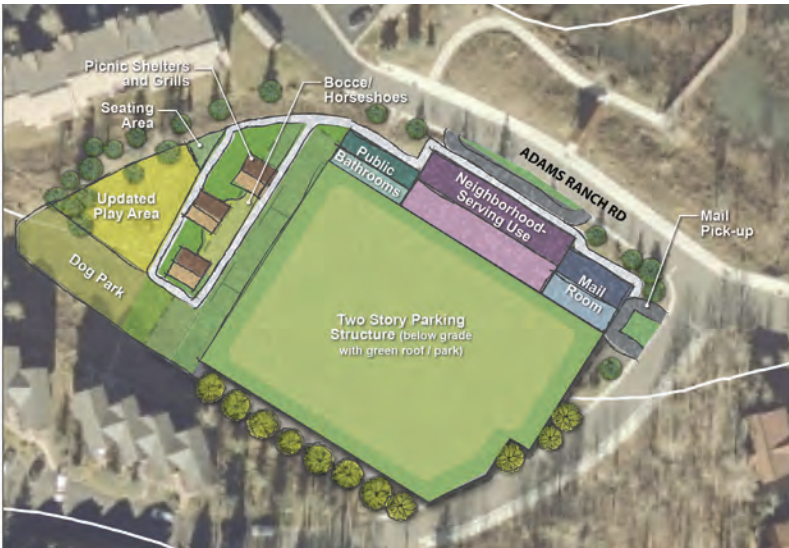
At grade: green roof/park expansion
