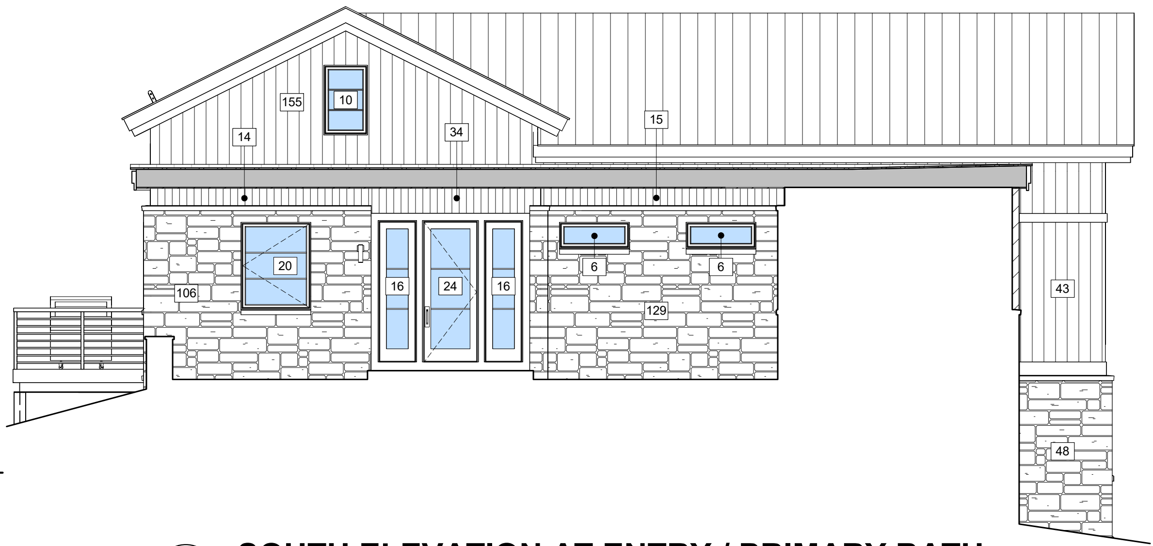
4 SOUTH ELEVATION AT ENTRY / PRIMARY BATH 3/16" = 1'-0"
